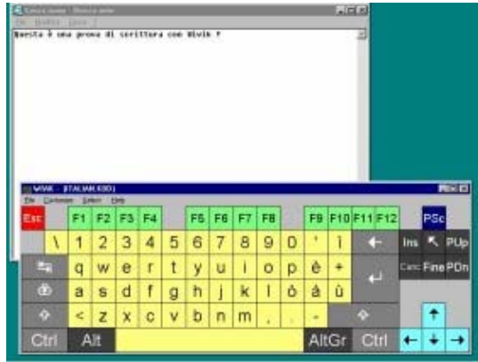
Figure 36 The layout of Wivik2, the user select the row and the column with a special input devices and the selected character appear on the Notebook application.
