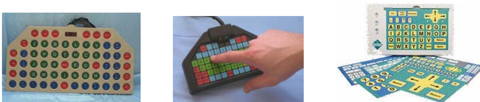
Figure 32 Examples of Expanded Keyboard, the WinKing Keyboard, Reduced Keyboard, the WinMini Keyboard and Reconfigurable Keyboard, the Intellikeys keyboard.
